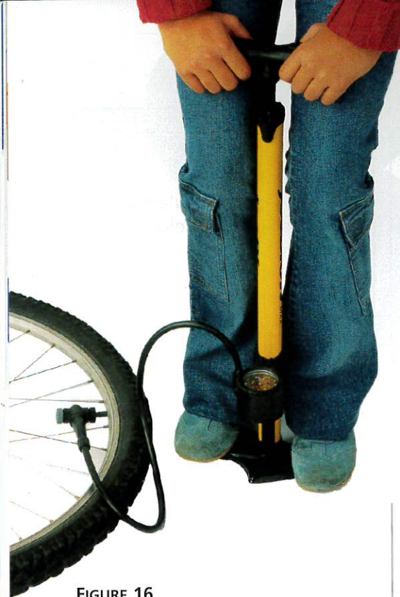
FIGURE 16 Inflating a Tire A bicycle pump makes use of the relationship between the volume and pressure of a gas.
