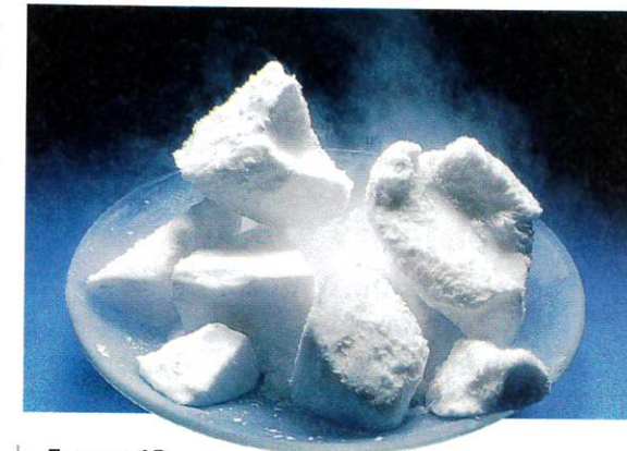
FIGURE 13 Dry Ice When solid carbon dioxide, called "dry ice," sublimates, it changes directly into a gas. Predicting If you allowed the dry ice to stand at room temperature for several hours, what would be left in the glass dish? Explain.
