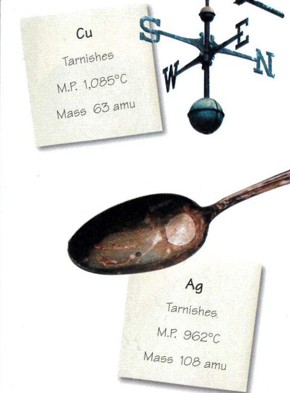
FIGURE 5 Metals That Tarnish A copper weather vane and a silver spoon both tarnish from contact with air.
